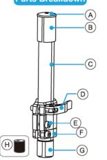
A. Top cap F. Head set tightening ring B.Stem clamping area G.25.4mm sleeve(white) C.Stanchion H.24.4mm sleeve(black) D.Quick release lever
