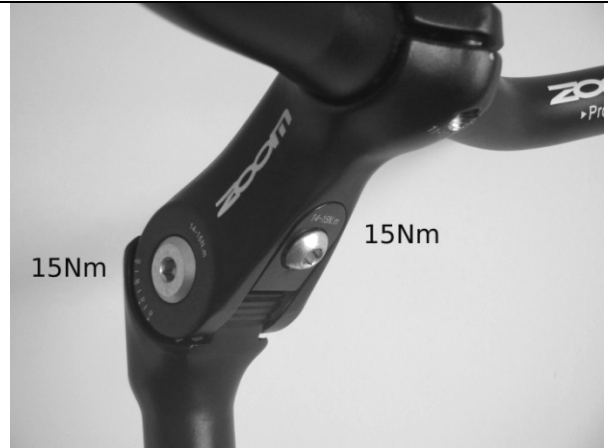
Figure 7 : Inclination of the stem, tightening torque
