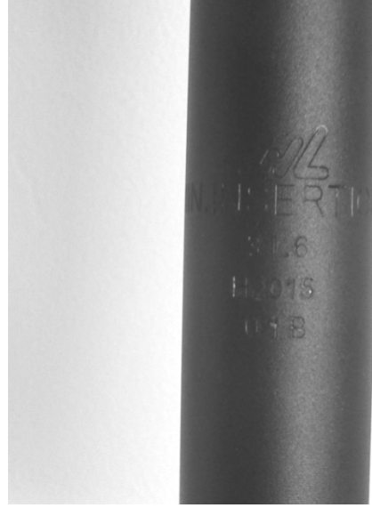
Figure 4 : Minimum sinking mark on the seat tube
