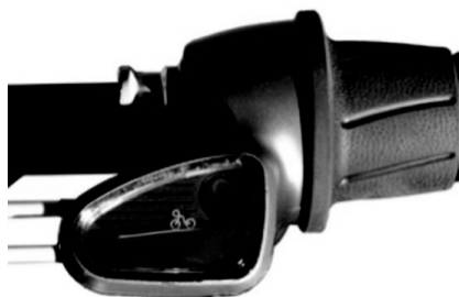
Figure 13 : In this position ('full overdrive'), the gear ratio is large. As the pictogram shows, this position is used when the ground is flat or downhill.
