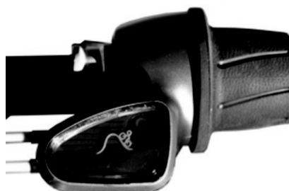
Figure 14 : In this position the gear ratio is small. This position is used whilst the terrain is uphill, when it becomes difficult to pedal while maintaining a consistent cycling cadence
