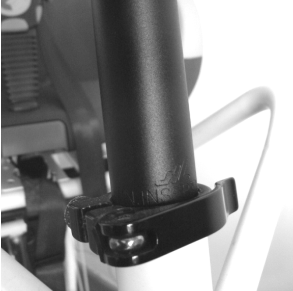
Figure 3 : Respect the minimum sinking of the seat tube
